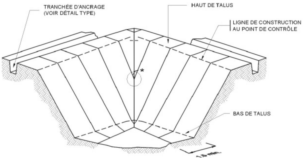
\* LA SOUDURE DES PANNEAUX NE COINCIDE PAS OBLIGATOIREMENT AU MÊME ENDROIT
